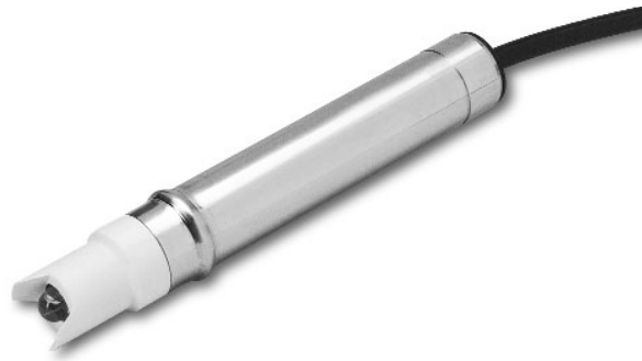
FIGURE 33. TUph Model 396 pH sensor (shown above) is offered without process threads. A compression fit, process connector is used on the sensor body and gives the user flexibility for insertion depths because the process connector can be tightened in various locations on the sensor body. Retractable sensors (a longer version of what is shown above) are also offered without process threads. This is so the sensor can be mounted through a ball valve.
